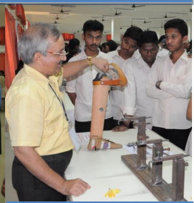
Terrain sensing Jaipur Foot by Prof. N.V. Deshpande & Prof. V.P. Ghodake, Kolhapur
