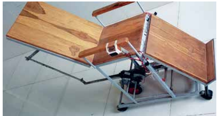
Wheelchair cum Stretcher with Multifold
